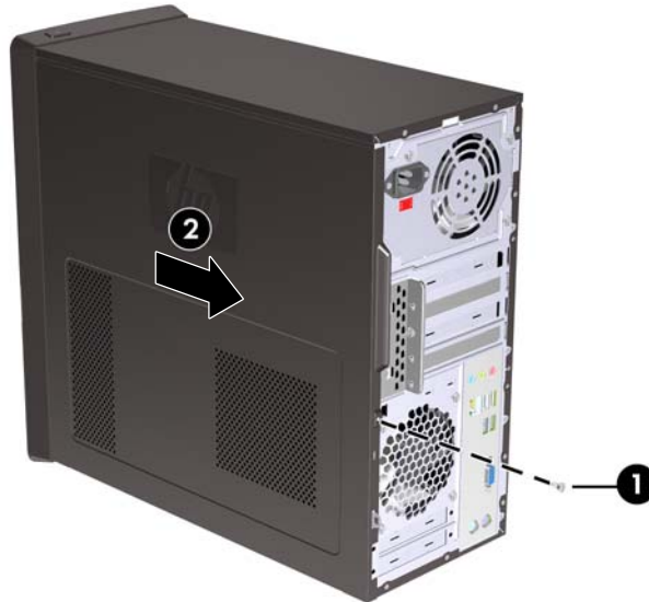
Figure 6-1 Removing the Computer Access Panel
